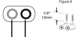
Typical speaker output using bare wire. Insert bare wire into the binding post and tighten.
